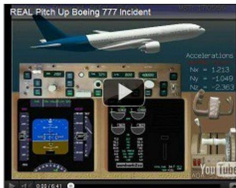
This animation shows a 3-D model of the aircraft and its motion and displays relevant information from the flight data recorder. It shows the information of the cockpit, including alarms, and it also shows the pilot's action on the flight controls, thrust levers and other levers and buttons, and various other data.
